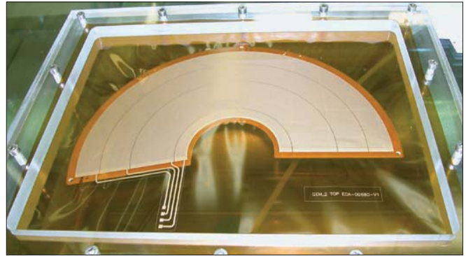
Each half-moon GEM foil for the TOTEM detector is 30 cm across.
