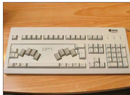
The new Braille keyboard has eight Braille keys, which allow typing in any language.
