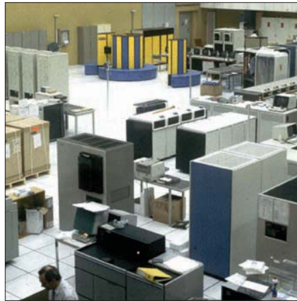
View of part of the Computer Centre in 1988. The CRAY X-MP/48 supercomputer can be seen in the background against the rear wall.
